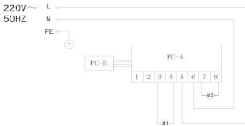
Note: M 1 --- compressor; M2--- stirring motor; PC-A --- Control panel; PC-B --- Operation panel; PE --- Grounding; L, N --- Power supply
